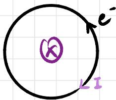
$$\begin{aligned} \mu &= IA \\ &= -\frac{e}{T} \pi r^2 \end{aligned}$$
