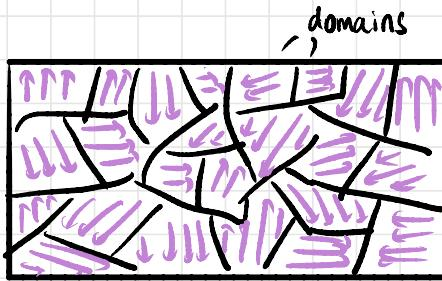
sintered polycrystalline material
